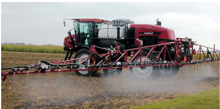
Figure 4. Ground sprayer utilizing pulse width modulation technology for drift reduction. (Courtesy: S. Bretthauer, University of Illinois)
