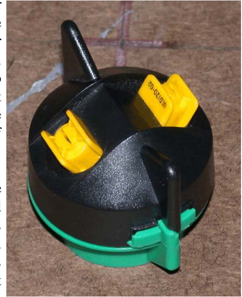
Figure 5. Twin nozzle cap with two individual nozzle tips. One set to spray forward in the direction of travel and the other set to spray backwards. (Courtesy: S. Bretthauer, University of Illinois)
