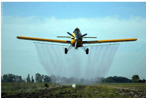
Figure 6. An aerial application with an aircraft set up to provide a uniform spray pattern. (Courtesy: D. Gardisser, University of Arkansas).
