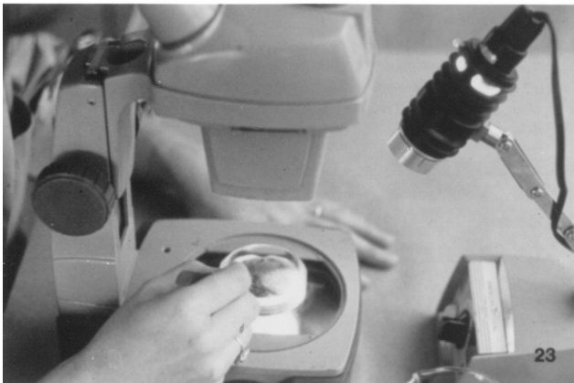
Figure 6. Count cysts at 15X using a dissecting microscope and an above-stage light source.
