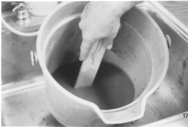
Figure 2. Mix 100 cc of soil with 2 quarts of water for 1 minute after all clods are broken up by hand.
