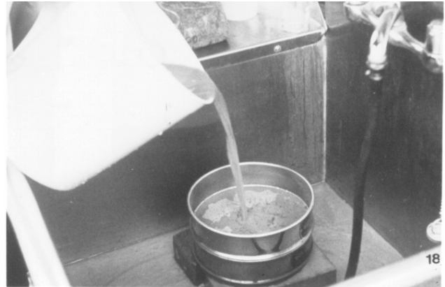
Figure 3. Pour liquid-soil suspension through a 20-mesh sieve nested on a 60-mesh sieve.
