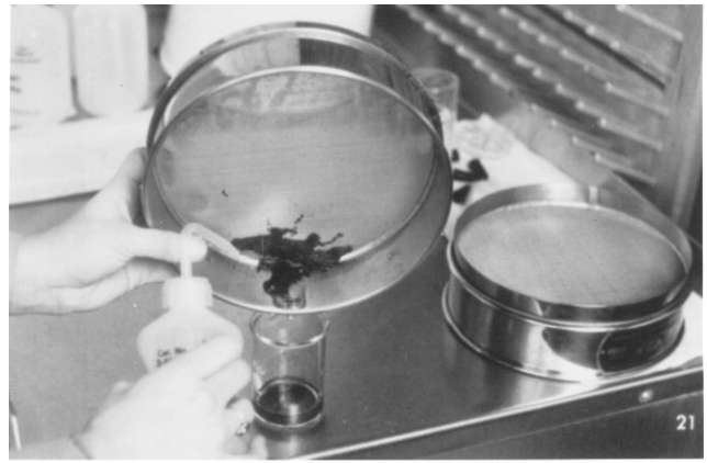
Figure 5. Backwash cysts into a beaker with a squeeze bottle.
