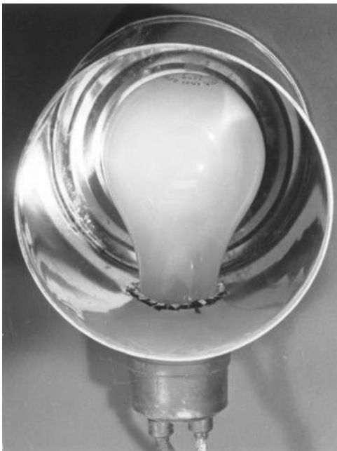
Figure 6. Homemade sulfur vaporizer used to control powdery mildew on greenhouse roses. A hole was cut through the side, near the bottom of a tin can, and a 60-watt light bulb inserted in the can and screwed into a suitable socket. Flowers of sulfur, placed in the bottom of the can, will be vaporized by the heat from the light bulb (Illinois Natural History Survey photo).
