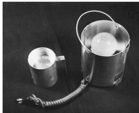
Figure 7. A commercially made sulfur vaporizer. The sulfur container (left) is over the light bulb and is secured by inserting the bracket into the clamp on the outer container (Illinois Natural History Survey photo).
