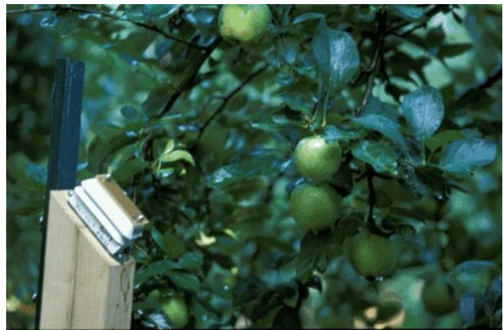
Figure 5. A Wetness/Temperature Logger under canopy of an apple tree.
