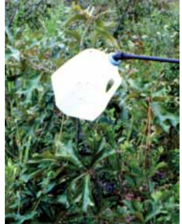
Spray shield from a used gallon milk jug (bottom removed and cap bored).
