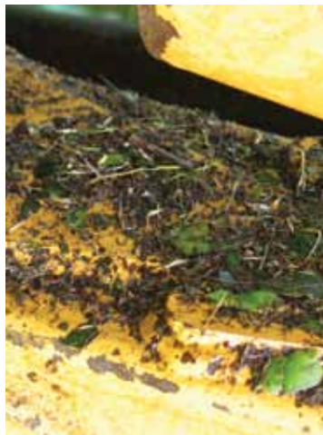
Excess grease traps seeds.
