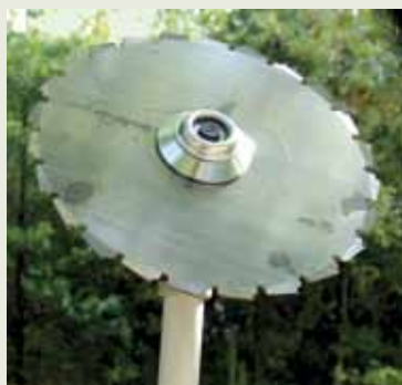
Brushsaw blade with chainsaw-like teeth.
