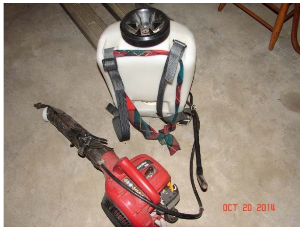
Backpack sprayer connected to a leaf blower for use as a mist-blower.
