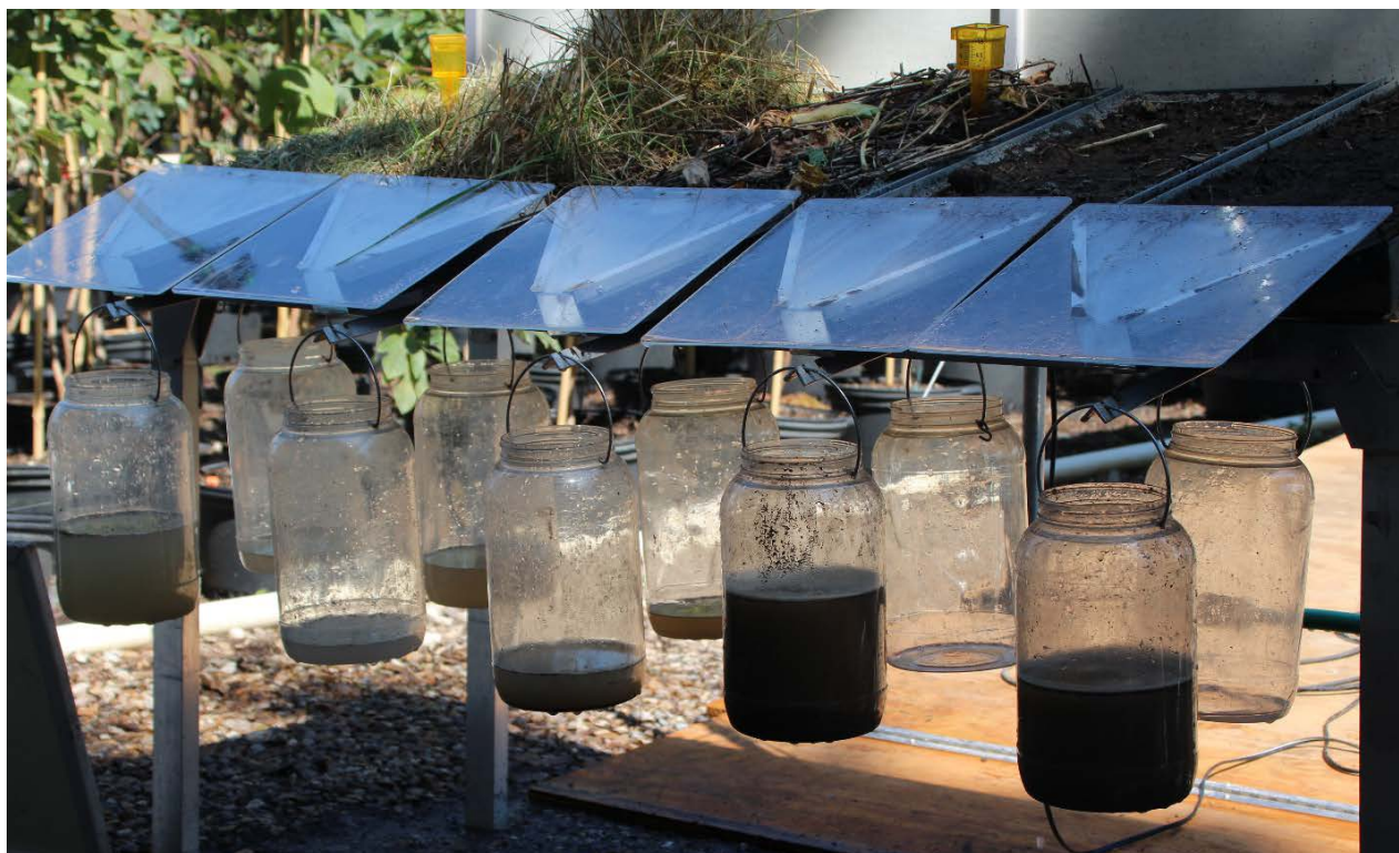
(L to R) Unmanaged pasture, Managed pasture, Heavy soil residue (no-till), Conventional tilled sample from a previous simulation (left to dry out), and Conventional tilled. The front row of jars represents runoff and erosion. The back row of jars represents water infiltration.
