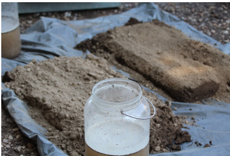
Relatively low water infiltration of conventional tilled soil following rainfall simulation.
